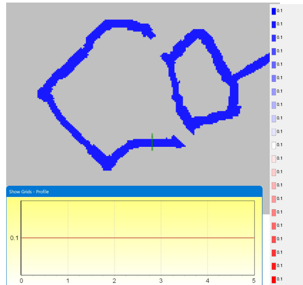
figure 2.29.2.2 IceWedgeUpperLimit (iwdegup) for the test basin (depth in cross section is at 0.1 m below surface for all calls on an ice wedge)
